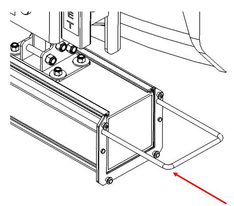
Slide the stainless steel pull handle back into the sleeve.
