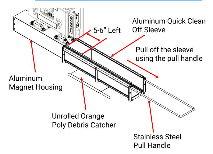
Pull the sleeve until there is just 5-6 inches of sleeve still over the magnet. It is highly recommended that the debris left on the sleeve be hand picked off the magnet.
